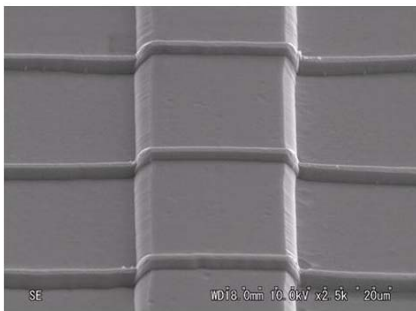
Fig. 1: Silica-based lines on a step structure
