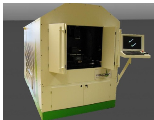
Figure 1 : Photo of the first fs workstation from IMPULSION company used for production (field of automotive industry)
