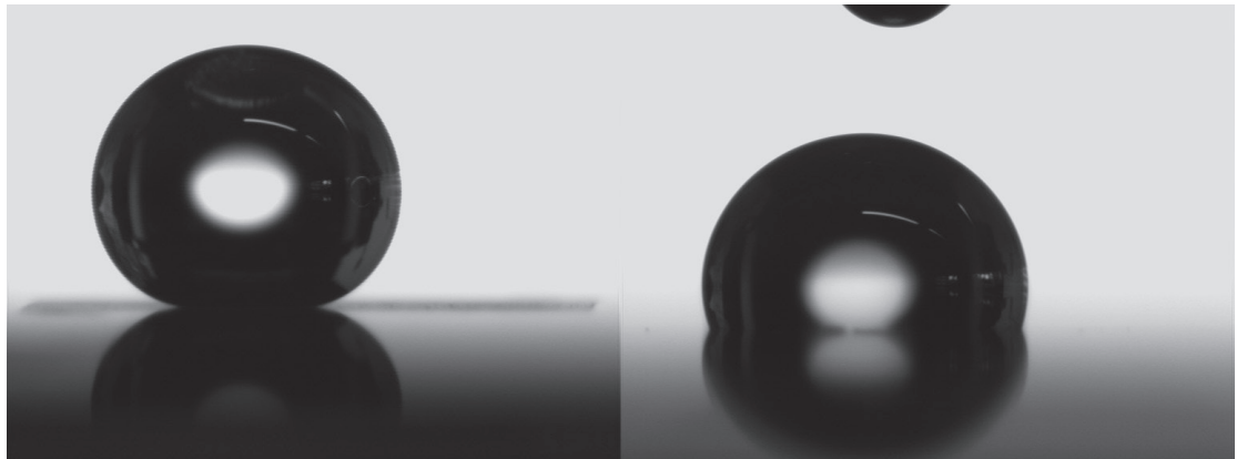
Figure 1. Effect of a laser texture on a stainless steel sample. The left drop on top of a laser micro structured surface exhibits a high contact angle; the surface on the right is smooth and wets the surface.
