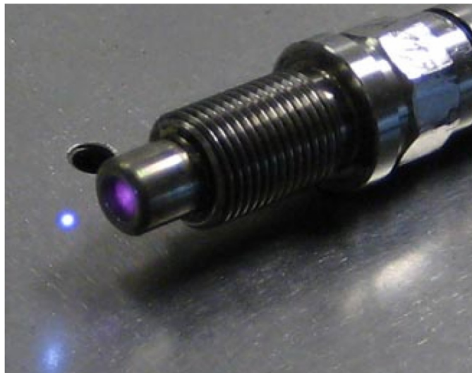
Figure 1 Plasma spark emitted from a laser spark plug developed at Vienna University of Technology. The heart of this device is a compact monolithic diode-pumped passively Q-switched Nd:YAG laser. Pulse duration ~1 ns, pulse energy >10 mJ.
