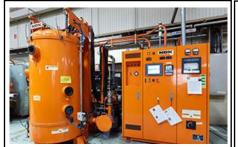
The ion nitriding method was invented by B. Berghaus, Germany, in 1932, and started to be put to practical use in German and Swiss companies around 1967. NDK developed the first ion nitriding instrument in Japan in 1973, and started manufacturing and contract processing services.
