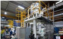
A radical nitriding system is configured of a furnace (vacuum-resistant, heat-resistant container), an electric heater, a vacuum evacuation device, a gas supply device, plasma and heater power supplies, an operating and control device and an exhaust gas processor.
