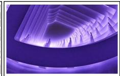
Plasma carburizing equipment makes use of the electrochemical reactions of the plasma from the DC glow discharge and thermal energy to form carbides on the surfaces of metallic materials to improve the mechanical strength.
