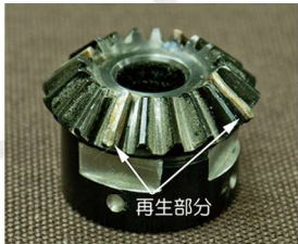
歯車補修 Repair of gear
