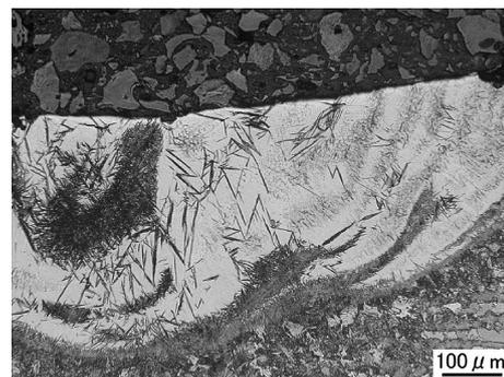
Fig. 5 Inhomogeneous microstructure of laser alloyed zone (paste thickness 0.25 mm, traverse speed 10 mm/s)
