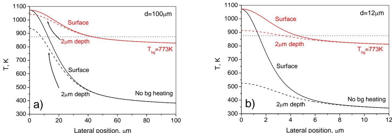
**Fig. 2** Calculated temperature profiles on the surface and 2  $\mu\text{m}$  below the surface for a 2-inch InP wafer irradiated by laser beams of 100  $\mu\text{m}$  (a) and 12  $\mu\text{m}$  (b) diameters. Laser power was adjusted for every simulation to reach the same maximum temperature. Horizontal line indicates the threshold temperature for which a 90-sec RTA induces no significant PL shift [3].
