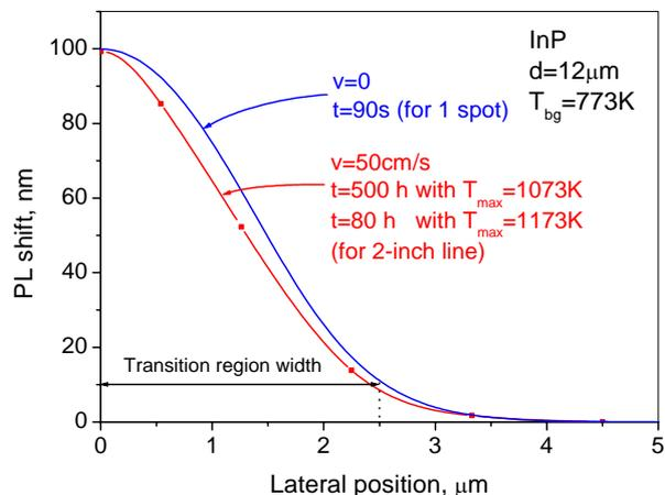
**Fig. 4** Calculated intermixing profiles for different scanning speeds.
