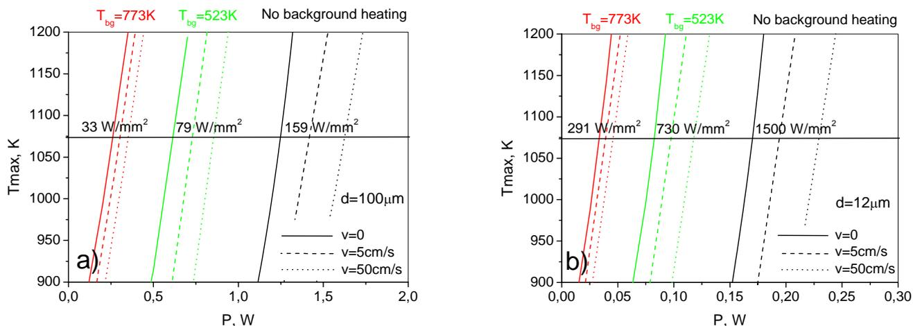
**Fig. 1** Dependence of InP sample surface temperature in the center of the beam ( $T_{\text{max}}$ ) on laser power for different scanning speeds and for beam diameters of 100  $\mu\text{m}$  (a) and 12  $\mu\text{m}$  (b). Power densities needed to achieve 1073 K with a stationary beam are shown in the picture. Horizontal line – temperature giving 100 nm PL shift in the InGaAs/InGaAsP QW microstructure following the 90-s RTA [3].
