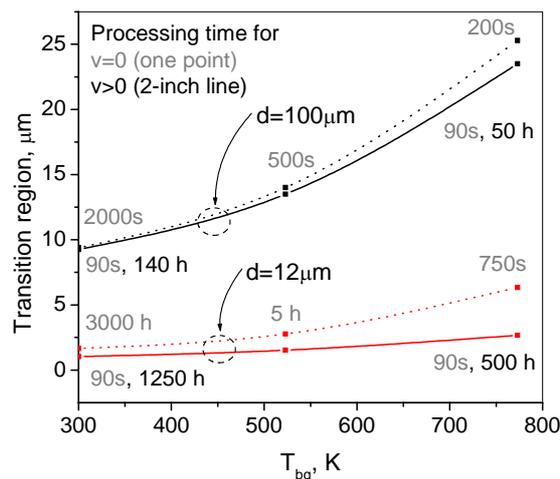
**Fig. 6** Transition widths and processing times to write a 2-inch line of the 100 nm bandgap shifted material at  $T_{\text{max}} = 1073$  K. The results at the surface (solid line) and 2  $\mu\text{m}$  below the surface (dotted line) have been calculated for 100 and 12  $\mu\text{m}$  beam diameters as a function of the background temperature.
