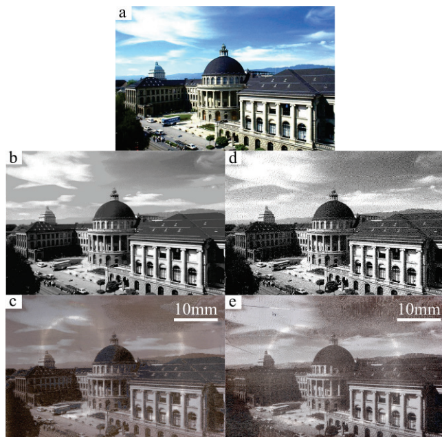
Fig. 8 Laser marking of a colored pixel image (a). Four grey level and dithering leads to the simulated graphic in (b) and the result on stainless steel in (c). Solely marking with black leads to different perception (d,e).
