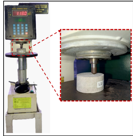
Fig. 5 Digital hardness testing setup with a magnified inset of the HRA measurement.
