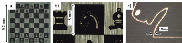
**Fig. 20** Black-marked image on stainless steel of (a) chess board, (b) and (c) zoomed in showing 10  $\mu\text{m}$  wide unmarked outline around the knight.
