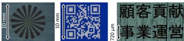
**Fig. 22** Images marked on silicon wafers in collaboration with A. Brand, Fraunhofer ISE. Laser used was Photonics Industries RX2 at 90 W power, 200 kHz repetition rate and peak fluence of 1.0  $\text{J}/\text{cm}^2$ .
