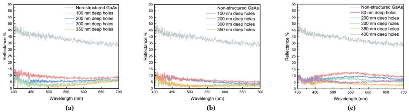
**Fig. 4** Comparative analysis of reflectance between bare GaAs substrates and GaAs substrates embedded with PhC structures **a)** 417 nm diameter and 500 nm pitch, ranging in depths from 100 nm to 350 nm; **b)** 440 nm diameter and 500 nm pitch, ranging in depths from 100 nm to 350 nm; **c)** 315 nm major axis, 305 nm minor axis and 365 nm pitch, ranging in depths from 80 nm to 400 nm.
