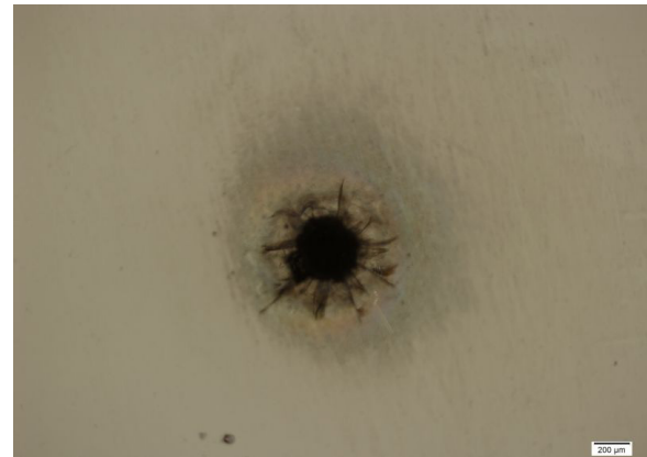
Fig. 8 \lambda=355 nm, d=+1 mm, 100 shots, absorption of stray laser radiation caused extensive damage
