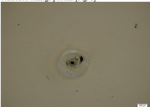
Fig. 7 \lambda=1064 nm, d=+1 mm, 100 shots, overheating the sample surface affects large area
