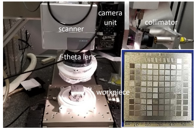
Fig. 4 Optical configuration of the LP system.
