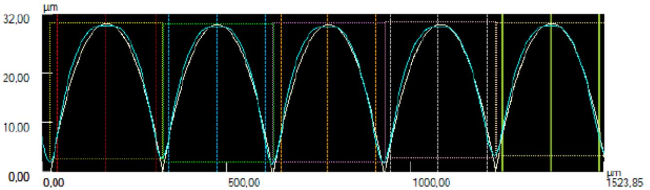
Fig. 3 Surface profile after polishing the surface from Fig. 1, measured average radius: 391 μm, standard deviation: 6,7 μm.
