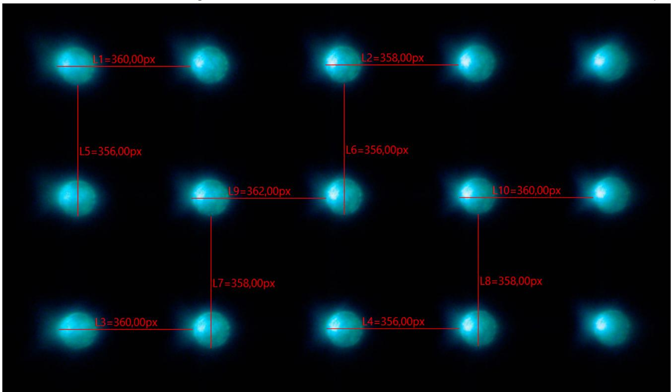
**Fig. 6** Image of the MLA foci in the camera. The structure of the cheap LED light source is visible in the foci. The size and spacing of the foci is constant within the measurement uncertainty.
