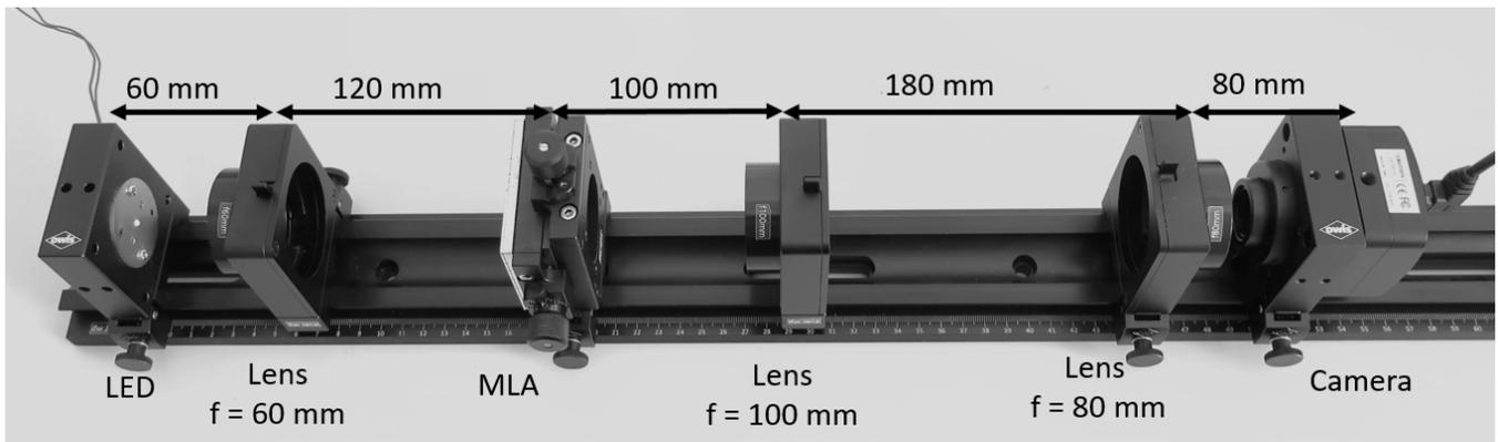
**Fig. 5** Optical test bench for the micro lens arrays, from left to right: light source (LED), collimation lens, MLA, 4-f-setup, camera
