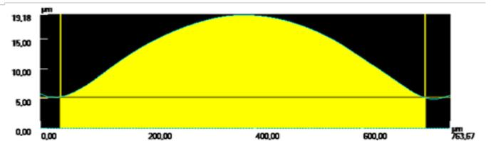
Fig. 4 Surface profile comparison with laser-polishing; Boro-float® 33, target radius: 3000 μm, target pitch: 500 μm; the lower part of the picture shows the diagonal cross sections
