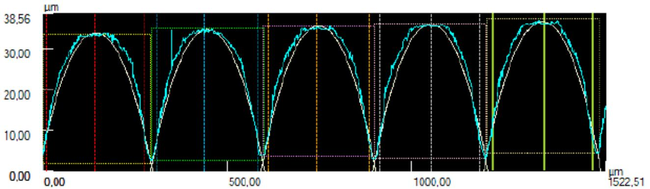
**Fig. 1** Surface profile after CO<sub>2</sub>-laser ablation before polishing; fused silica, target radius: 350 μm, measured average radius: 358 μm, standard deviation: 4,4 μm; the white curve is a manually fitted spherical contour to calculate the radius. The maximum deviation from the contour is about 8 μm.
