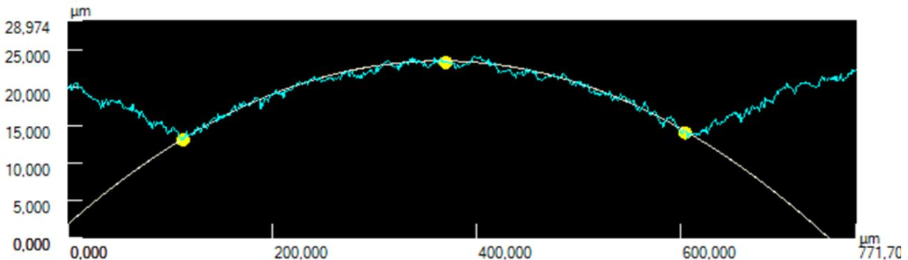
**Fig. 2** Surface profile after USP-laser ablation; Boro-float® 33, target radius: 3000 μm, measured radius: 3075 μm
