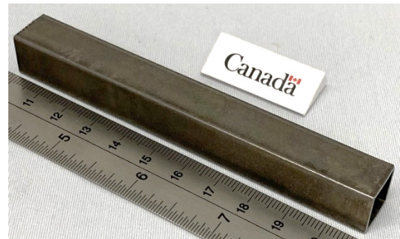
Fig. 2 DLD-fabricated tubular thin wall sample.
