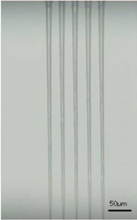
Fig. 5 Side view of micro-vias fabricated by excimer laser ablation in 500 \mu\text{m} thick glass. Upper side is irradiation surface.
