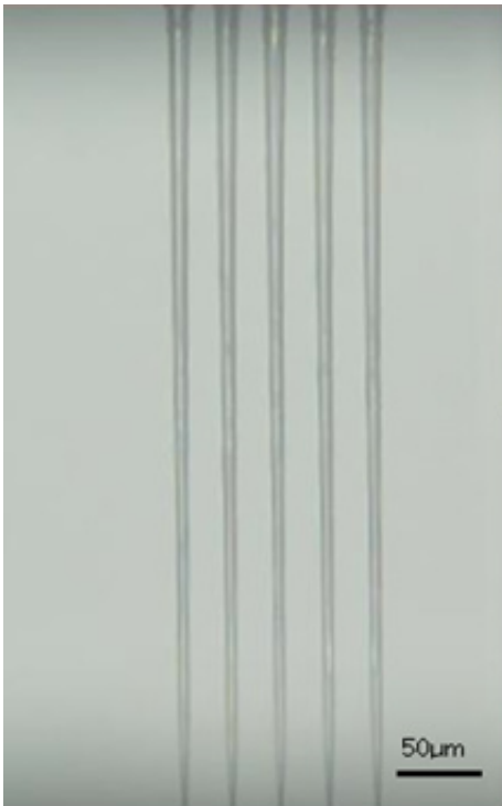
Fig. 5 Side view of micro-vias fabricated by excimer laser ablation in 500 μm thick glass. Upper side is irradiation surface.
