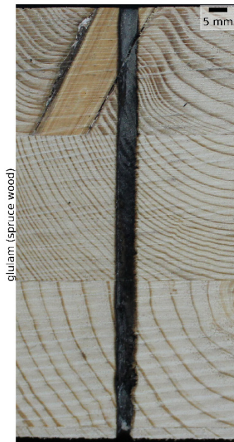
Fig. 11 Cross section of a sample for USP deep drilling with knot-hole within 120 mm thick glulam. The carbonized borehole wall and the density changes in the lamellas are visible.
