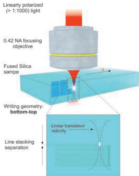
**Fig. 1** Writing geometry and components used in the experiments.
