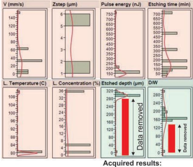
**Fig. 3** Density plots of the varied parameter values (top) and acquired results (bottom). Only the channels that have fully etched are displayed and where the D/W ratio is larger than 150 (see text.).
