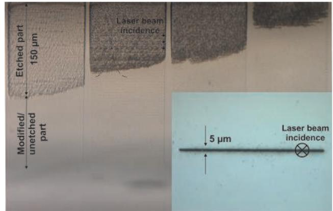
**Fig. 2** Images of partially etched out channels after an etching session. A profile view is displayed. Each channel was inscribed with different parameters. The inset shows the entrance of the channel.
