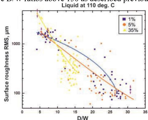
**Fig. 5** Measured surface roughness values plotted against the possible D/W ratio. One can notice that different roughness is achievable for different D/W ratio values. The solid lines are eye-guides illustrating that lower roughness typically is achievable with higher D/W ratios.
