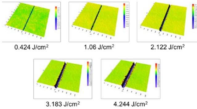
Fig. 8 3D contour profile of grooves ablated with 50 ns pulse duration at different laser fluence.
