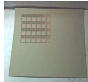
Fig. 11 Example of customised silver film produced using laser ablation technique.
