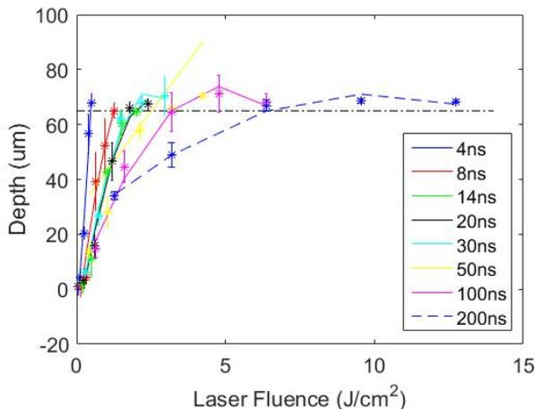
Fig. 10 Groove depth variation with different laser fluence and pulse duration with a single pass.
