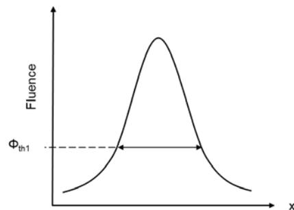
Fig. 7 Schematic diagram illustrating the correlation between the Gaussian spatial distribution of the laser fluence with the ablation width.
