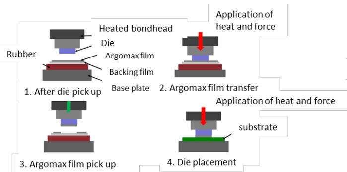
Fig. 1 Die Transfer Film (DTF) process and die placement using a Die Bonder equipment [1].
