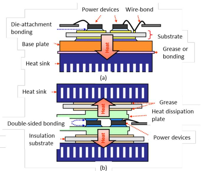
Fig. 2 Power module schematic of single and double-sided cooling [2].
