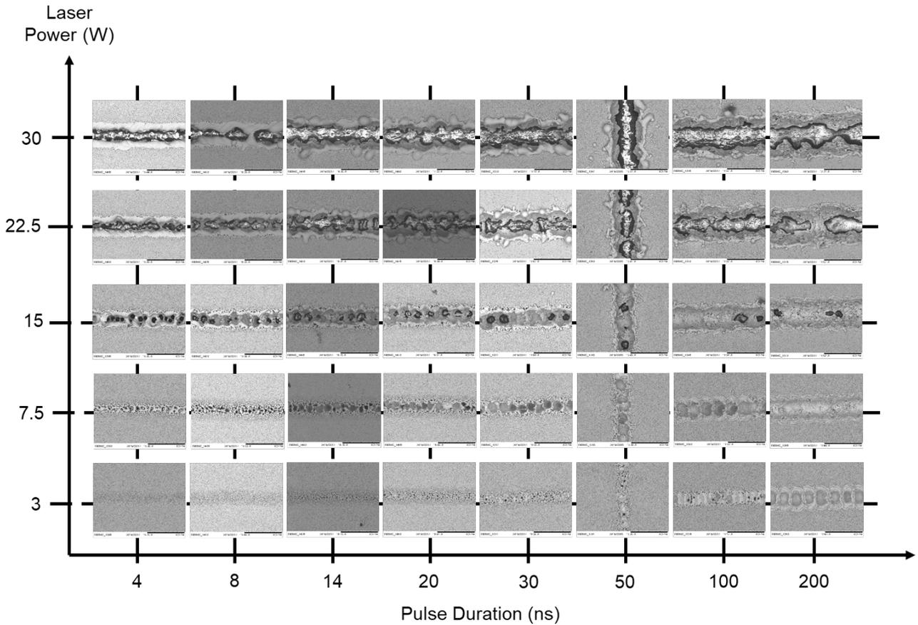
Fig. 5 SEM images of laser ablated grooves with different laser power and pulse duration with a single pass.
