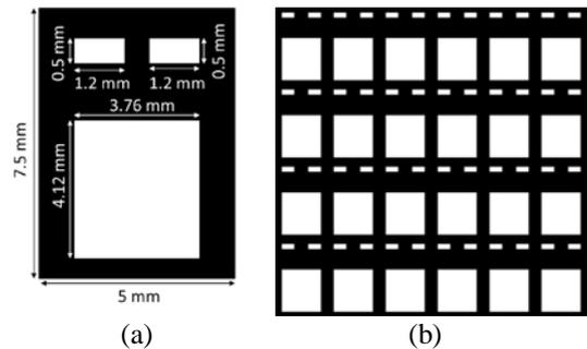
Fig. 4 (a) Dimension of the unit cell for the power module. (b) Array of unit cells for mass production.
