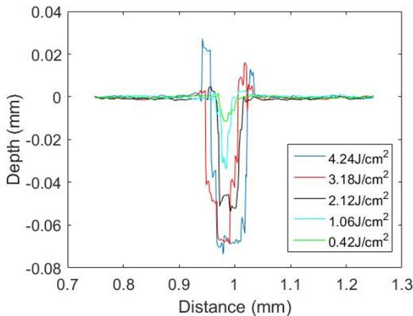
Fig. 9 Cross section profiles of grooves ablated with 50 ns pulse duration at different laser fluence.
