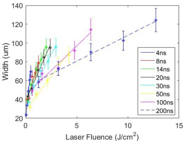
Fig. 6 Groove width variation with different laser fluence and pulse duration with a single pass.
