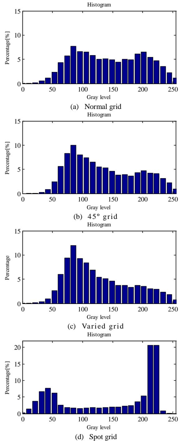
Fig. 2 Corresponding histograms of four subtypes of speckle patterns produced with laser scribing.
