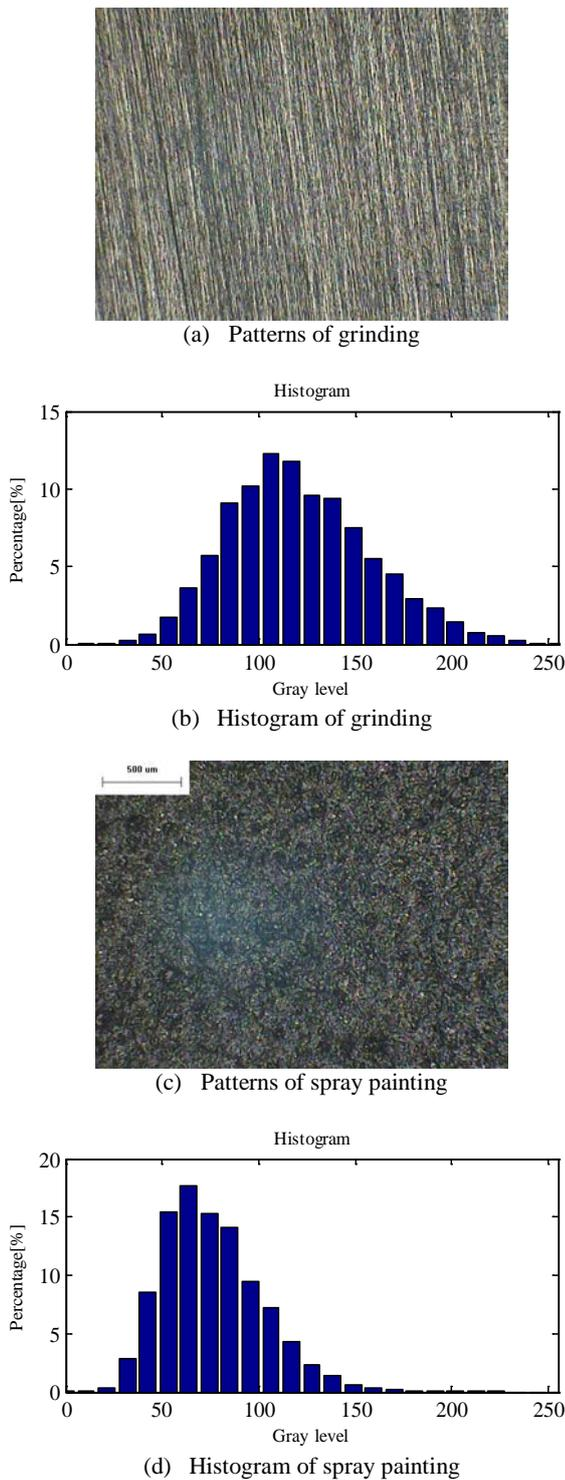
**Fig. 3** Speckle patterns produced with grinding and spray painting, and their corresponding histograms.
