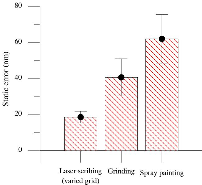
Fig. 4 Static error estimation of each speckle patterns without movement.
