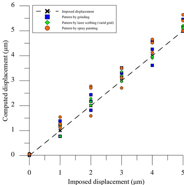
Fig. 5 Displacement field computed using DIC and real imposed displacement (an increment of 1 µm).
