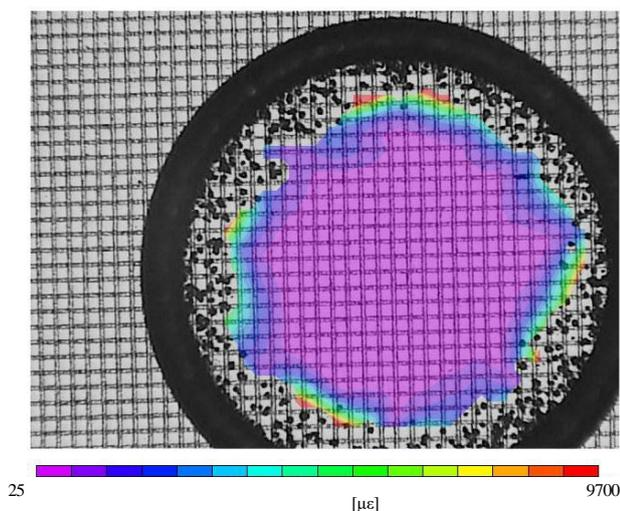
Fig. 7 Additional thermal strain analysis of laser scribing.
