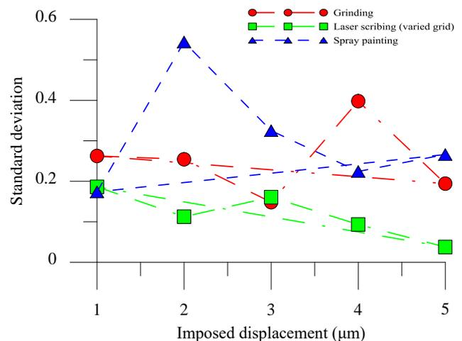
Fig. 6 Standard deviation of measured horizontal displacement for the five speckle patterns using 61 × 61 pixels subset (along the horizontal line of the image).
