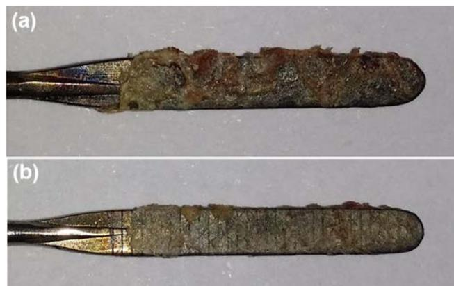
**Fig. 7** Liver tissue adhesion on the electro-surgical knives: (a) Original blade without bionic shark skin; (b) The blade with bionic shark skin.
