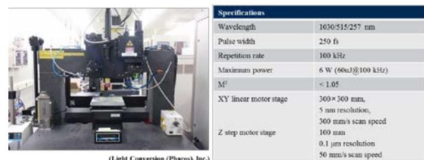
Fig. 1 Femtosecond laser micro-machine system
