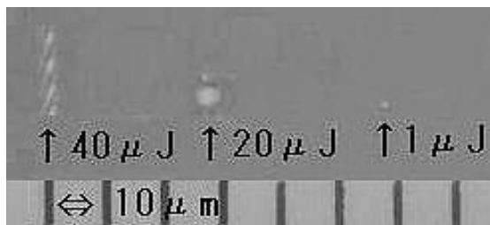
Fig. 3 The change in the processing shape by the difference of the pulse energy of the laser
