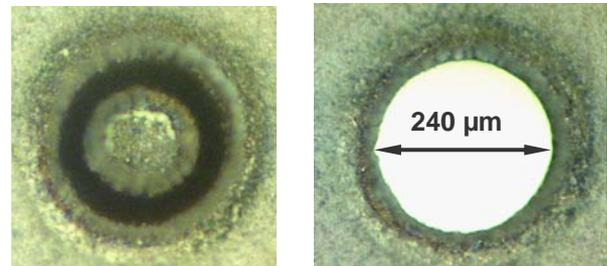
**Fig. 5** Microscope pictures of two different stages after laser trepanning of a 500  $\mu\text{m}$  thick tungsten sample at a circular displacement of 200  $\mu\text{m}$ : Processing time from left to right: 5s and 10 s.
