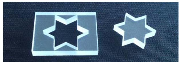
**Fig. 4** Examples of laser glass trepanning. Top: 1.2 mm through-hole in 48 mm thick glass cube (with a special taper in the middle). Below: star shape cut out of a 3 mm thick soda-lime glass.
