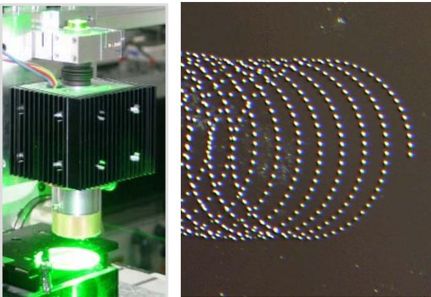
**Fig. 3** Laser trepanning and cutting of glass. Right: microscope picture of glass substrate marking the very beginning of the trepanning cycles
