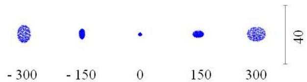
**Fig. 2** Simulated beam intensity distribution (ZEMAX) for a defined optical trepanning system design, given for different positions (-300, 150, 0, +150, and +300  $\mu\text{m}$ ) relative to focal point. Note: the airy disk for a laser beam at focus (not shown) is ca.  $20 \mu\text{m}$ .
