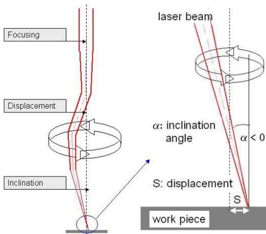
**Fig. 1** Illustration of the beam path along the LMTB trepanning system: The beam propagates through (stationary) focusing optics and the rotating displacement & inclination optic set-up. The right picture depicts a magnified view near focal point with definition of inclination angle and beam displacement at the work piece
