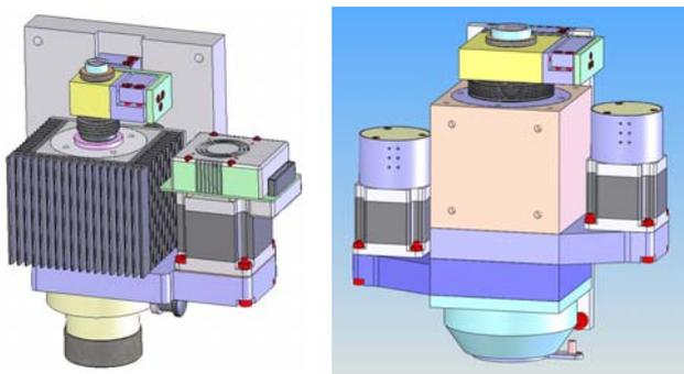
**Fig. 6** CAD illustrations of completed laser trepanning systems for solving universal drilling problems, i.e. control of drilling diameter and taper.
