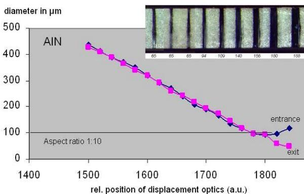
**Fig. 7** AIN ceramic through-hole diameter of entrance and exit hole versus relative position of the displacement optics. The insert above right depicts a microscope image after the cross-section polish of the AIN sample.
