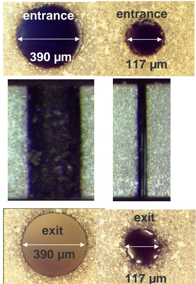
**Fig. 8** Microscope images of two cylindrical through holes, 390 and 117 mm, in an 1 mm thick AIN sample: entrance hole (top), cross-section (middle) and exit hole (bottom). Note: the scale for the cross-section differs from the entrance and exit hole.
