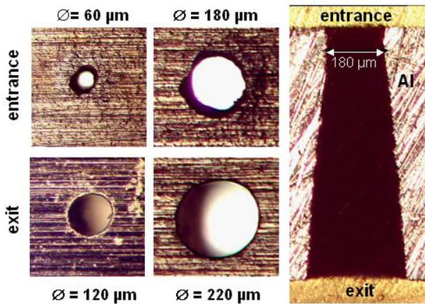
**Fig. 9** Microscope images of reversed tapered through holes in Al-metal sample, 600 (left and middle) and 800 $\mu\text{m}$  (right cross section) thick.
