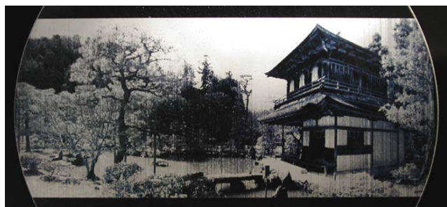
Fig. 15 FLIP image of Ginkakuji (Silver Pavilion) in Kyoto machined onto sapphire surface.
