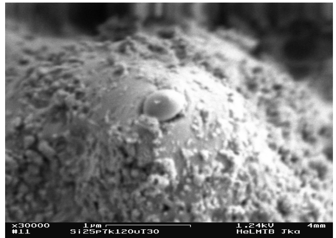
Fig.3. SEM image showing a nanocolumn formed on top of the conical microspike of silicon.
