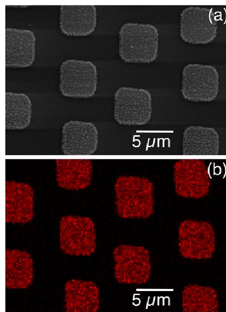
**Fig. 3** SEM-EDX analysis of an array of laser decal transfer silver voxels. (a) SEM image and (b) corresponding SEM-EDX element mapping of the  $Ag_L$  line. Red indicates the presence of silver while dark color indicates its absence outside the regions covered by the voxels.
