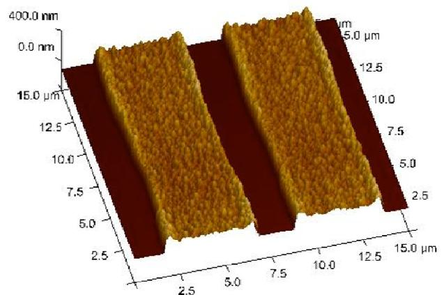
**Fig. 6** AFM image showing two  $5$   $\mu\text{m}$  wide silver lines with a  $2$   $\mu\text{m}$  gap made by laser decal transfer.
