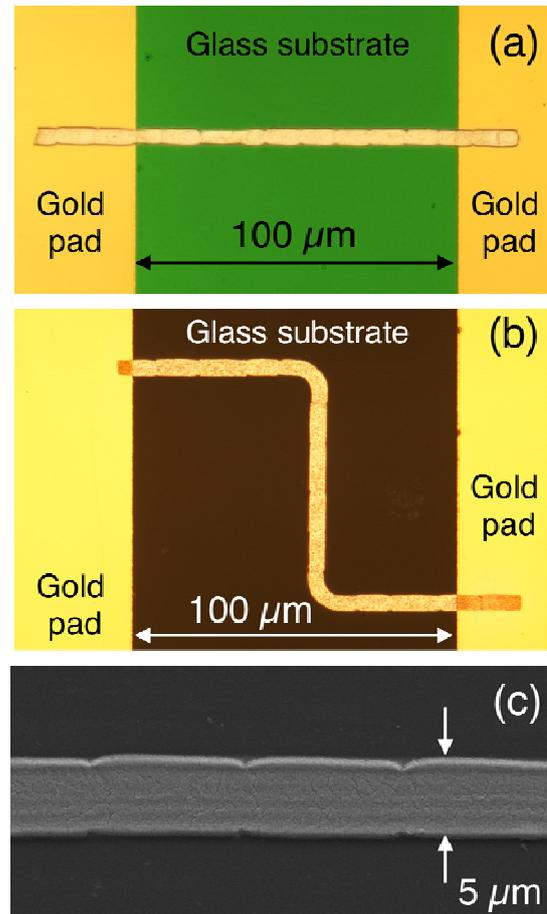
**Fig. 5** Optical micrographs showing conductive silver lines made from laser decal transferred individual voxels across gold pads on glass substrates. (a) Line made from  $15$   $\mu\text{m}$  long  $\times$   $5$   $\mu\text{m}$  wide adjacent voxels; (b) line made by combining the rectangular voxels from (a) with corner shaped ones; (c) SEM image showing a section from the line in (a). Note the continuous pattern across voxels.
