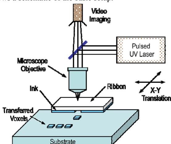
Fig. 1 Schematic diagram showing the basic components of the laser direct-write system used for laser decal transfers.
