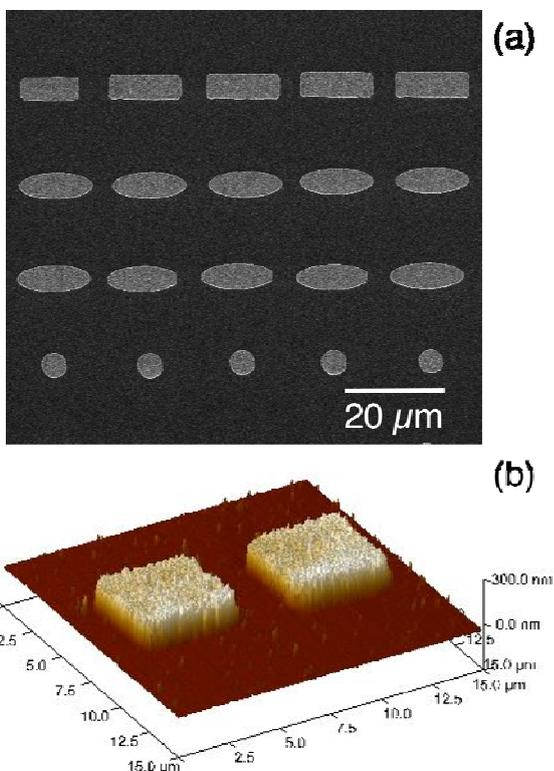
**Fig. 2** Examples of laser decal transfer of silver nanoink on a silicon substrate. (a) SEM image showing the transfer of rows of voxels using different apertures. (b) AFM image from two square voxels showing the high thickness uniformity and sharp edge definition of each transfer.
