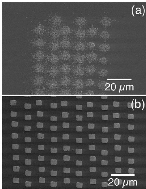
**Fig. 4** SEM image showing laser transfers under identical conditions for (a) low viscosity ( $\approx 10$  cP) silver nanoink and (b) high viscosity ( $\approx 100,000$  cP) silver nano-particle suspension.
