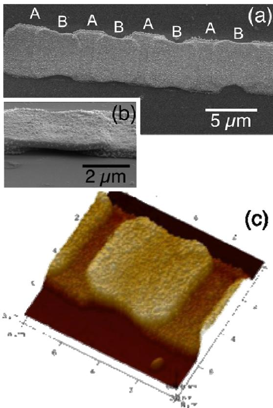
**Fig. 7** (a) SEM showing a two-layered line made by laser decal transfers of  $5\ \mu\text{m} \times 5\ \mu\text{m}$  voxels on silicon (A: 1<sup>st</sup> layer, B: 2<sup>nd</sup> layer). (b) Glancing angle SEM image showing one of the top layer voxels across the two voxels below. (c) AFM image showing one of the top layer voxels bridging the gap formed by the first layer with minimum sagging and distortion.
