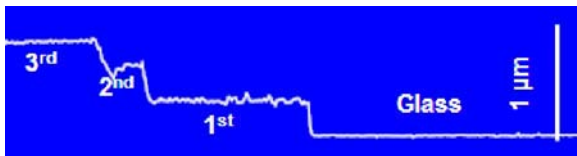
Fig. 7 Profile of multi-step structure fabricated by subsequent ablation of non-annealed ITO nanoparticle layers.
