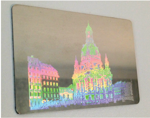
Fig. 7 Processed image of the Church of our Lady (Dresden, Germany) on stainless steel (50 x 75 mm 2 ) using DLIP- \mu FAB system.
