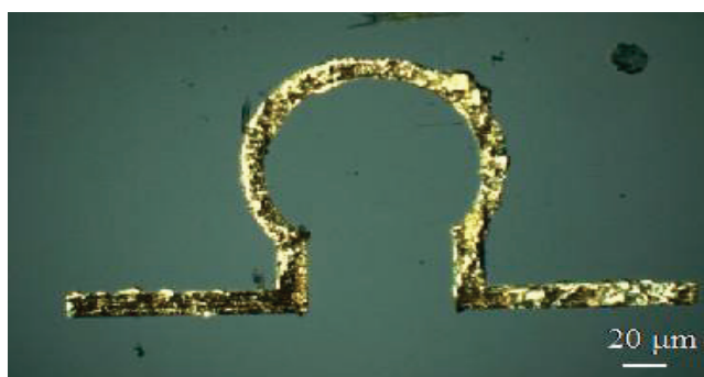
Fig.4. The optical micrograph of an “Ω” shaped gold microelectrode.
