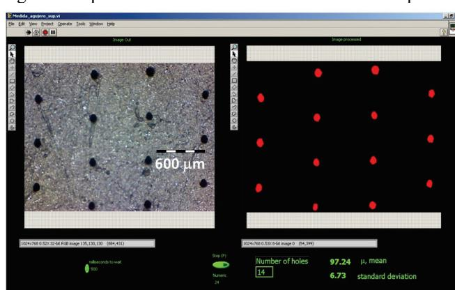
**Fig. 7** Front panel of the developed software for measuring the diameters of the holes automatically and obtaining statistical information.
