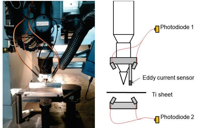
**Fig. 2** Left: Laser head. Right: Diagram of the sensors used for controlling the process
