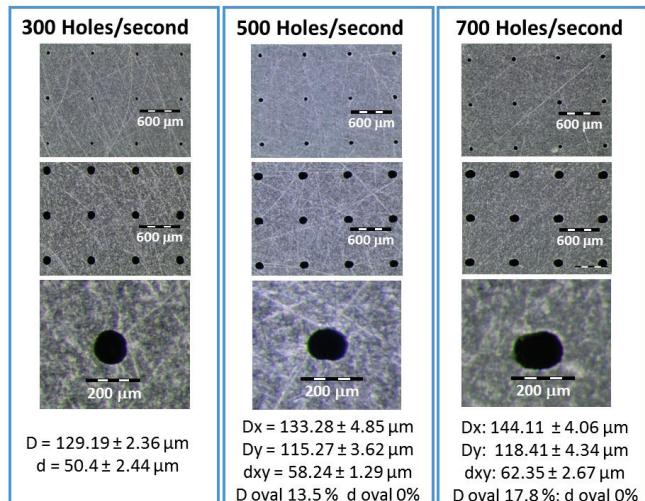
**Fig. 8** Measurements of micro-holes produced at rates of 300, 500 and 700 holes/s. Pictures at the top row: Exit side. Pictures at the central row: Entrance side. Pictures at the bottom row: detailed view of a hole at the entrance side
