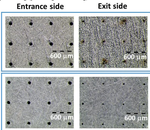
**Fig. 4** Pictures of the sample micro-drilled at lens position 0 mm before and after post-processing. Upper row: sample after laser micro-drilling. Lower row: sample after polishing and etching
