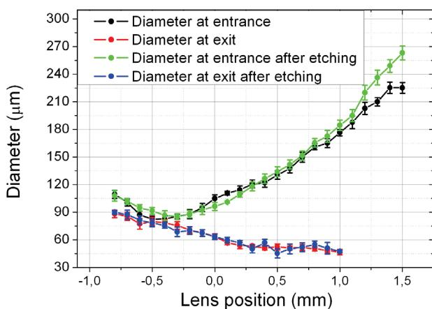
**Fig. 3** Diameter of the micro-holes at the beam entrance and exit as function of the lens position. The curves after mechanical and chemical post-processing for removing burrs and debris have been also added
