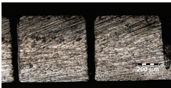
**Fig. 6** Cross-section of a group of micro-holes. No alpha-case layer formation has been detected in the hole walls.
