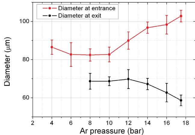
**Fig. 5** Diameter of the micro-holes at the beam entrance and exit as function of assist gas pressure.
