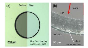
Fig. 2 a) Microscopy images of processed hole before and after cleaning in the ultrasonic bath. Dark regions are microscope artifacts due to dust redeposition and hole taper. b) Sideview of the processed hole shows that the dust is redeposited mainly at the rear side of the hole.
