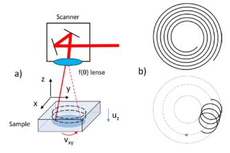
Fig. 1 a) Schema of experimental setup for the bottom-up drilling. b) Patterns for individual layer ablation: spiral (top) and "wobble" (bottom)
