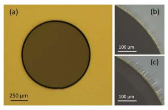
Fig. 4. a) Optical transmission microscopy image of drilling at 1MHz, 2.8 J/cm<sup>2</sup>, NA=0.09, t<sub>p</sub>=300fs, scanning speed 1 m/s, vertical translation speed 100  $\mu$ m/s. Residual stresses and internal defects may be revealed in cross-polarized light illumination in the case of b) optimal exposure c) and when overexposure of incident surface takes place.
