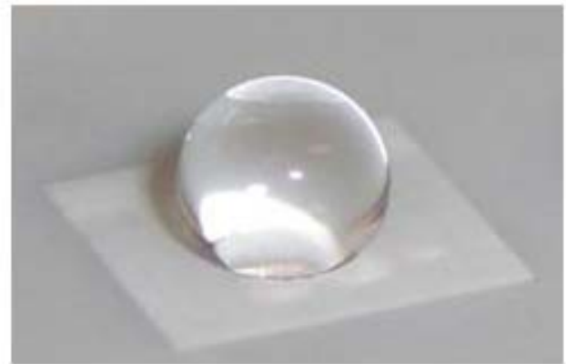
Fig. 6 Water droplet on the superhydrophobic surface of Teflon. White part is the laser machined area. (machined pitch:10 μm, contact angle:140 deg.)
