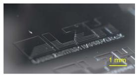
Fig. 6 LZH logo produced with 2D patterning in UV curable PDMS by UV-LDW
