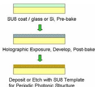
Fig. 1 Process Steps for Laser Nanofabrication.
