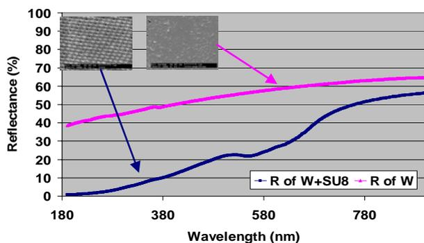
Fig. 4 Comparison of reflectances with and without tungsten deposited on SU8 photonic crystal.
