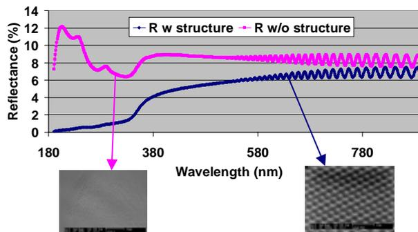
Fig. 3 Reflectances of SU8 surface with and without photonic crystal structure.
