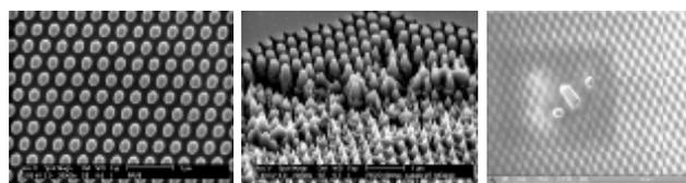
**Fig. 8.** SEM images of 2D structures in positive photoresist (left), nano pillars and spires etched on Si (center), and nano FIB machining to create functional defects (right).
