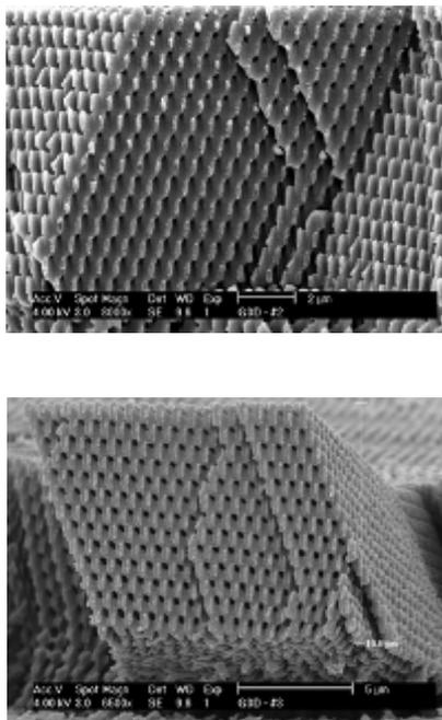
Fig. 2 Cross-sectional SEM of three-dimensional photonic crystal structures.
