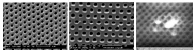
**Fig. 9.** SEM images of 2D structures in negative photoresist (left), nano holes etched on Si (center), and nano FIB GIS deposited W to selectively create functional defects (right).
