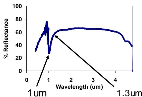
Fig. 5 Top view of 3D photonic crystal in SU8 (above) and a reflectance spectrum showing a photonic bandgap (below).
