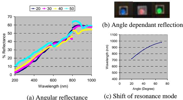
**Fig. 6** Angular dependence of reflectance from the tungsten filled SU8 photonic crystal and the shift of resonance modes with angle.
