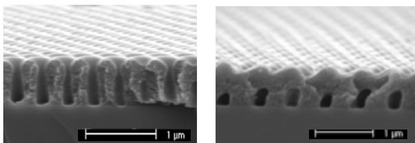
**Fig. 7** 2D structure (left, pitch of 360 nm) and 3D structure (right, pitch of 600 nm).
