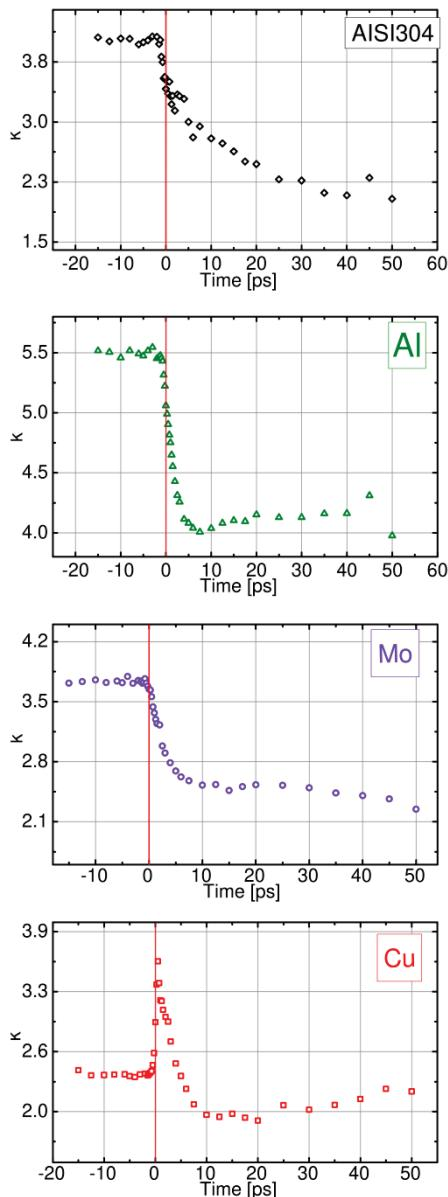
Fig. 2 Change in the extinction coefficient  $k$  for the four metal targets AISI304, Al, Mo and Cu at probe time steps from -15 to 50 ps
