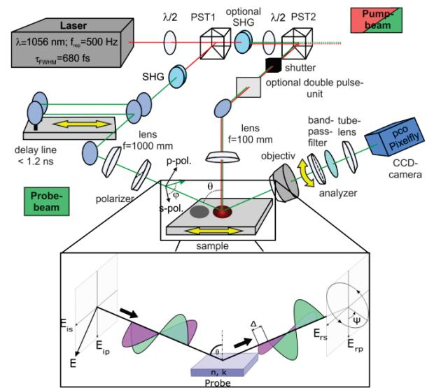
**Fig. 1** Pump probe ellipsometry setup for the determination of the transient change in complex refractive index for each metal target. The box at the bottom illustrates the change in polarization after reflection from the metal surface
