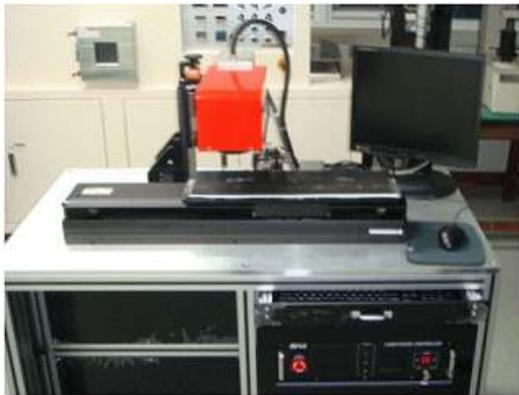
Fig. 6 Photo of one-axis stage–two-axis scanner on-the-fly system
