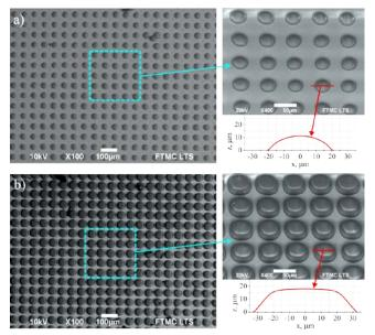
**Fig. 2** SEM micrographs at different magnification and profiles of structures produced via the four-beam interference lithography using a different laser irradiation dose: a)  $\sim 4.7~J$  (the average laser power  $\sim 0.47~W$  and laser exposure time 10 s); b)  $\sim 27.9~J$  (the average laser power  $\sim 0.93~W$  and laser exposure time 30 s). The period is  $\sim 60~\mu m$ . The structures in right SEM images are tilted by 34 deg.
