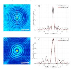
**Fig. 5** Intensity distributions of the generated beams formed using different types of the structures: a) I; c) II; at the distance of 200  $\mu$ m (a) and 350  $\mu$ m (c) from the sample and the comparison of the transverse intensity profiles taken along the white line (black curves) with the numerical fit of the Bessel beam intensity distribution when  $k_{\perp}$ =1.15 (b) and  $k_{\perp}$ =0.65 (d) (red lines). The scale bars represent 20  $\mu$ m. [26]
