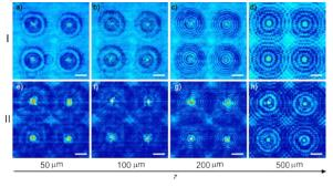
**Fig. 4** Beams intensity distributions exiting from the different type of the structures (type I (a,b,c,d), type II (e,f,g,h) in the transverse plane, at different distances from the tip of the structures:  $50 \mu m$  (a,e);  $100 \mu m$  (b,f);  $200 \mu m$  (c,g);  $500 \mu m$ (d,h). The scale bars represent  $20 \mu m$ . [26]
