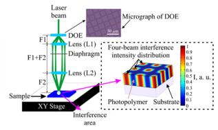
Fig. 1 The four-beam interference lithography experimental setup.
