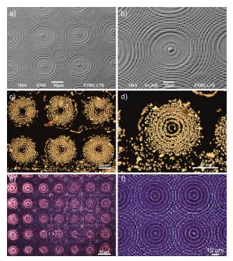
**Fig. 9** Structures fabricated by using microaxicon-like structures as the beam-forming element: a-b) SEM images of structures polymerised in SZ2080 (thickness  $\sim 10~\mu m$ ) tilted by 30 deg; c-d) optical microscope images of structures ablated in the thin gold film ( $\sim 20~nm$ ); e-f) optical microscope images of modified surface of the thin-film ink coated glass.
