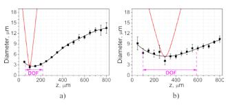
**Fig. 6** Alteration of the central spot diameter of the generated beams (black curves) by using a different type of structures: a) I type; b) II type. The black dots – the measured central spot diameter along z. The red curves show theoretically estimated divergence of the Gaussian beam when the beam waist diameter is  $2.4 \mu m$  (a) and  $5.4 \mu m$  (b). DOF means the depth of focus.
