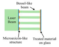
Fig. 8 The principle utilization scheme of microaxicon-like structures in the material treatment.
