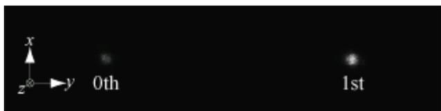
**Fig. 3** Schematic of diffraction pattern. The fabricated grating with the period of  $3\ \mu\text{m}$  and thickness of  $150\ \mu\text{m}$ . The fabrication energy was  $1.0\ \mu\text{J}$  and translation speed of the filament was  $1\ \mu\text{m/s}$ .
