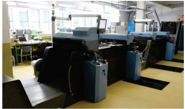
Fig. 8. Lasersonic® printing machine in the lab. The first printing unit is for absorbing ink, like black, the other three for non-absorbing inks like magenta, cyan and yellow. Printing units can be exchanged within a few minutes to vary between different inks or ink sequences.
