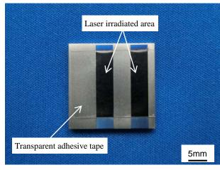
Fig.2 Appearance of the specimen after laser alloying.
