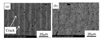
**Fig.3** SEM images of the surface of the specimen. (a)The area directly laser irradiated without the adhesive tape. (b)The laser-alloyed zone with the adhesive tape.
