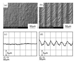
**Fig.5** Surface topographic images ((a), (b)) and surface profiles ((c), (d)) of the laser-alloyed zone by SEM.
