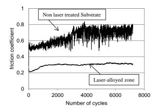
Fig.8 Friction coefficient during wear testing.
