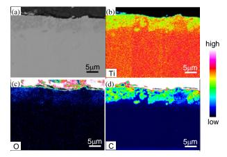
**Fig.7** Results of EPMA plane analysis of the laser-alloyed zone using nanosecond laser.
