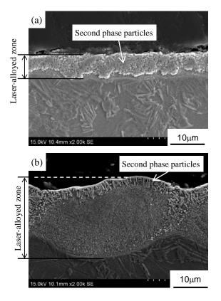
**Fig.4** SEM images of the cross section of the specimen after laser alloying using (a) nanosecond laser (Average power 10W, Scanning speed 100mm/s, Scanning pitch 15μm) (b) CW laser (Power 30W, Scanning speed 150mm/s, Scanning pitch 50 μm).
