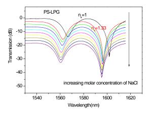
**Fig. 8** Transmission spectra of a typical PS-LPG sensor in aqueous solution containing increasing concentration of sodium chloride (from top to bottom).
