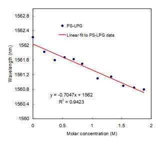
Fig. 9 Plot of peak wavelength of a typical PS-LPG versus molar concentration of sodium chloride solutions.
