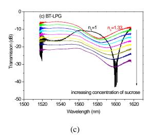
Fig. 6 Transmission spectra of a typical (a): LPG;(b): PS-LPG; and (c): BT-LPG sensors in aqueous solution containing increasing concentration of sucrose (from top to bottom).
