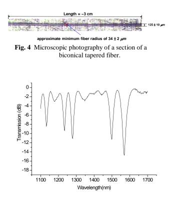
Fig. 5 A typical transmission spectrum of a PS-LPG.
