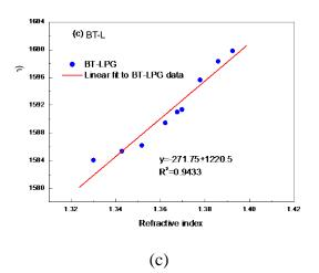
Fig. 7 Plots of peak wavelength versus RI of the sucrose solution for a typical (a): LPG; (b): PS-LPG; and (c): BT-LPG sensors in aqueous solution containing increasing concentration of sucrose.
