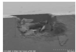
Fig. 3 SEM image of coarse microstructure fabricated with two consecutive strokes laser focused on the surface of PMMA slide.
