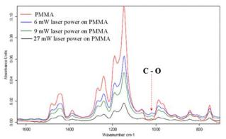
Fig. 7 Spectra of PMMA polymeric surface treated with different laser energies.
