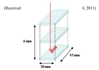
**Fig. 2** Schematic illustration of micromixer. We decomposed the sketch into three parts. The red arrow indicates the laser beam.
