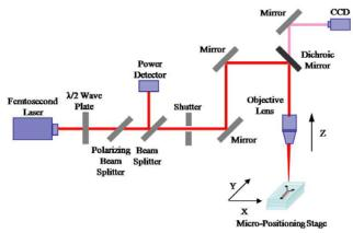
**Fig. 1** Schematic illustration of the experimental setup for fabrication of microstructures.
