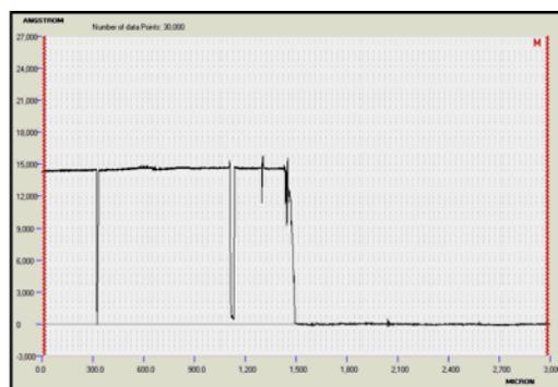
**Fig. 8** Profile graph generated during the measurement of the thickness of an unbaked polymer film
