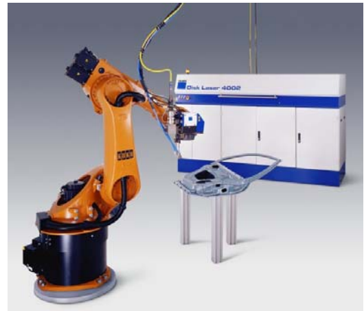
Fig. 4 Robot with a programmable focus optic (PFO) connected to the thin disc laser via fiber.
