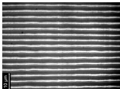
Fig. 6 Cr grating on the glass substrate formed by self-organization under the nanosecond laser irradiation. Energy density 1.9 J/cm 2 , pitch 0.3 μm.
