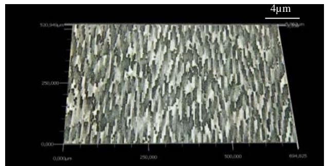
Fig. 29 in stainless steel engraved diffractive structure, pixel size: 4µm, depth 1,4µm, 30steps
