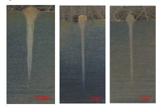
**Fig. 3** Cross sections of bead-on-plate welds on stainless steel X5CrNi 8-10 (AISI 304) (YW50; 240 mm focal distance).
