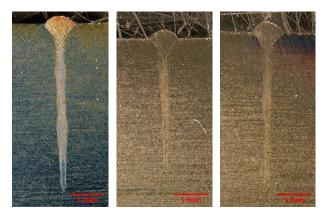
**Fig. 5** Cross sections of bead-on-plate welds on stainless steel X5CrNi 18-10 (AISI 304) (YW50; 500 mm focal distance). **Left:** laser power: 3 kW; processing speed: 5 m/min; penetration depth and width: 5.1 mm / 0.24 mm.
