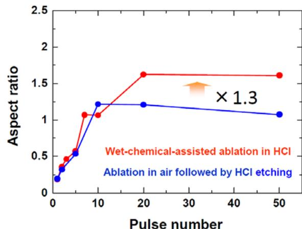
**Fig. 5** Aspect ratios as a function of pulse number for the wet-chemical-assisted ablation (red closed circles) and two-step processing (blue closed circles).
