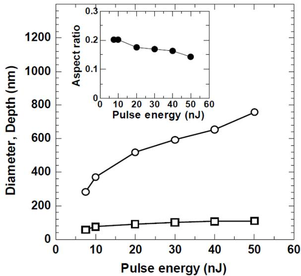
**Fig. 1** Pulse energy dependence of diameter (○) and depth (□) in ablation craters formed by single-pulse irradiation using wet-chemical-assisted fs laser ablation. Inset is the variation of the aspect ratio (●).
