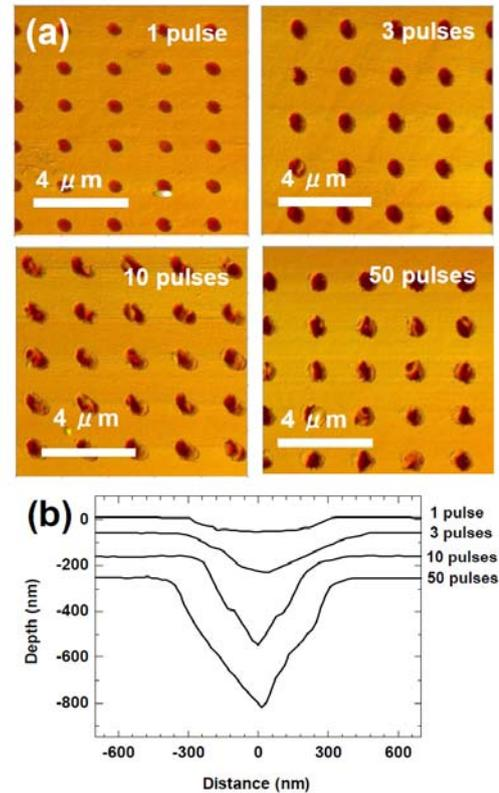
**Fig. 2** (a) AFM images of nanohole arrays formed by multi-scan irradiation method using wet-chemical-assisted ablation in HCl solution at a pulse energy of 10 nJ for various pulse numbers, and (b) cross-sectional profiles of nanoholes for each pulse number.
