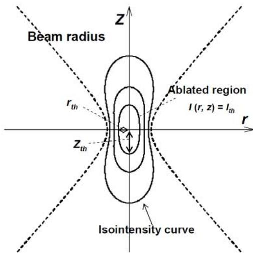
**Fig. 6** Beam radius (dotted line) and isointensity curves for various intensities (solid lines). In particular, the isointensity curve for the ablation threshold intensity represents the ablated region formed by the multi-scan irradiation technique.
