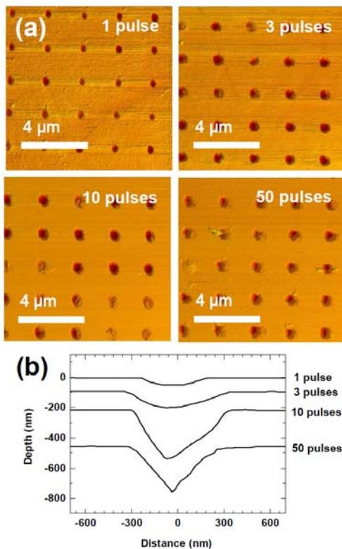
**Fig. 3** (a) AFM images of nanohole arrays formed by multi-scan irradiation method using two-step processing method at a pulse energy of 10 nJ for various pulse numbers, and (b) cross-sectional profiles of nanoholes for each pulse number.
