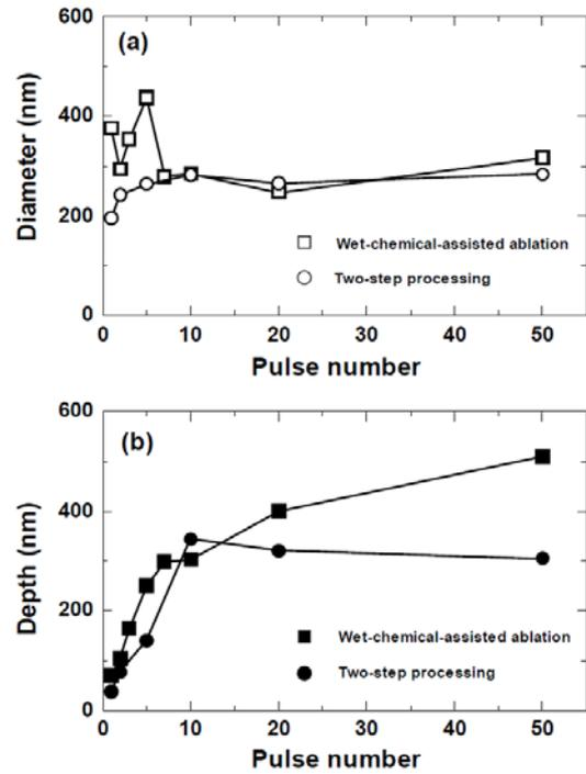
**Fig. 4** Pulse number dependence of (a) diameter and (b) depth of nanoholes formed using the multi-scan irradiation method in the case of wet-chemical-assisted fs laser ablation (□ and ■) and two-step processing (○ and ●).
